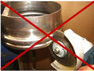
**DO NOT** cut BFM™ Spigot and re-size before installation.
