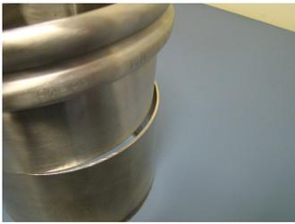
Size fitting to pipe. Pipe circumference may need to be expanded or reduced to suit the BFM™ Spigot.
