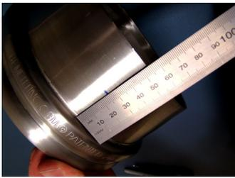
Avoid (if possible) cutting the tail down. If it is necessary to shorten the tail, do not cut the tail down any more than 25mm. Welding, any closer than 25mm to the head, could result in welding shrinkage effecting the tolerance of fit between the flexible connector cuff into the BFM™ fitting.
